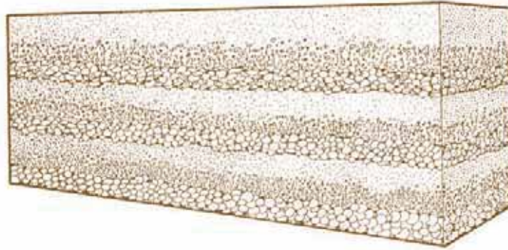
Figure 6.2. A cross-section through three graded sedimentary beds. In each bed, the larger particles are at the bottom, and the smaller particles at the top. Courtesy of Mark Ford.
