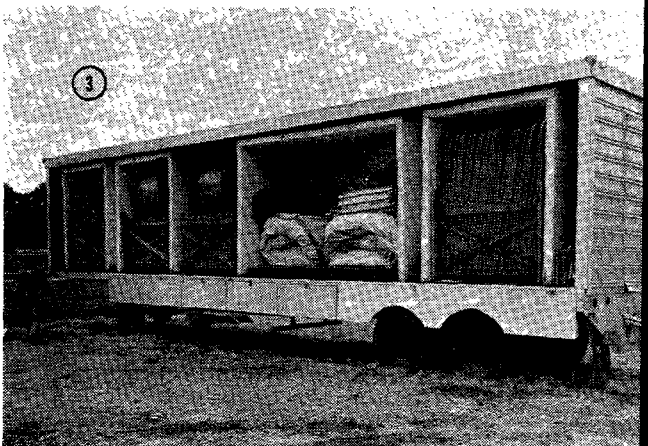
(1) Doorways are not disassembled, but are loaded as units by fork lift. (Lift is rented from local lumber yard.)
